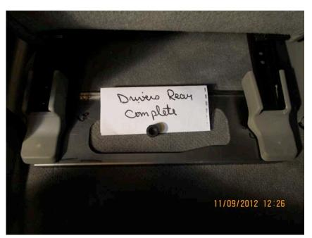
Grab the larger 1 piece bracket. Lay it down in the rear area. Now line up the 2 rear OEM holes and finger tighten the 2 remaining factory bolts.
