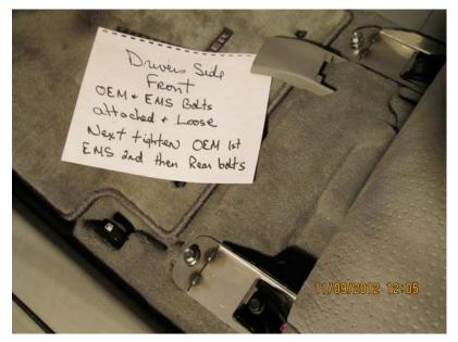
Lay down the 2 black brackets inside your vehicle and line up the 2 OEM hole locations. The bracket bends will face inward.
