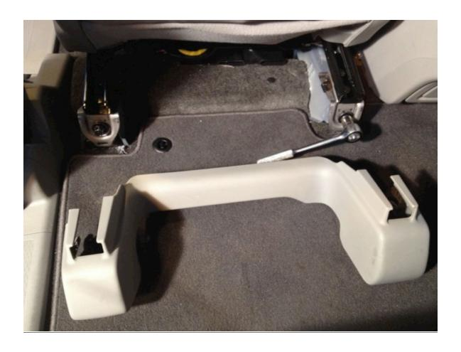
Now un-bolt the front factory seat foot from the seat chair on the front inner locations (2 bolts). The 2 bolts are under the factory foot.
