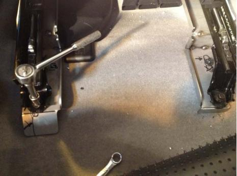
Step 10-Press seat lever and slide seat to the most up front position. Go to back seat and screw down secure the remaining 4 rear bolts.
