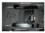
Lay down the two black ExtendMySeat brackets inside your vehicle so the four factory holes align. Slightly tighten the two front factory bolts into the two front ExtendMySeat bracket holes. The one M10 bolt provided will be used on the hole facing the inside of the vehicle in the rear of bracket B. Align the last remaining rear hole with the rear hole in bracket A.
