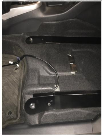
5. Re-place seat on EMS brackets and thread 3/8-16 bolts into the seat track mounts, after all 4 are started in their threads, tighten all bolts.
