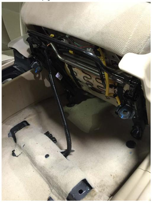
4. Bolt brackets to bottom of seat using supplied 3/8" bolts, locate brackets to floor and hand thread factory bolts to floor
